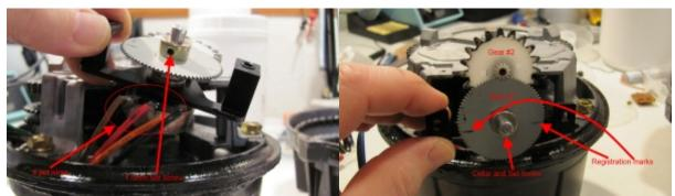
Step 8: Carefully slide the pot with Gears #1 and #2 (items #45 and #47) out from the Gear Box Plate, and pull the wires and the pot assembly out into the open. Note the registration marks I made on Gear #1. This may be helpful to you during reassembly.
