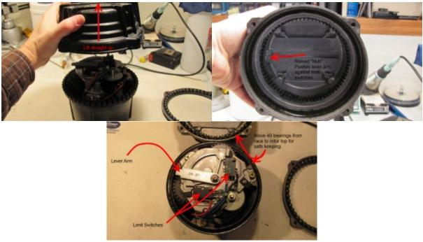
**<u>Step 5</u>**: Carefully lift the top of the rotor straight up to disengage the gears, then tip it over top down onto the table top.
