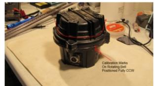
Step 1: Operate the rotor to its fully CCW position.
