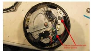
Step 12: Slide the pot assembly back onto the Upper Gear Box Plate (item #33). Carefully guide the teeth of Gear #2 (item #47) into the mating gear inside the gear box. Don't mesh the gears too much, allow a small amount of play between gears. Your registration marks on Gear #1 (item #46) should line up very closely with the edges of the Upper Gear Box Plate. Install the two screws and snugly secure the pot assembly to the Upper Gear Box Plate, but do not over tighten!
